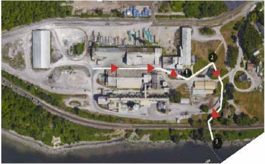
1. Oil Storage Building 2. First Settling Pond 3. Outfall 4. Storm and Cooling Water Flow (white line showing direction)
