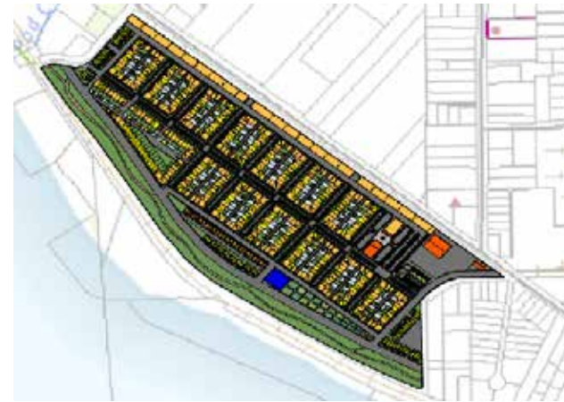
Right: Aerial view of the site development. Type of development is represented by the colors of buildings: public use (blue), single-family homes (orange), multi-family housing (yellow), park (green), commercial (red), and Additional Housing Units (light blue).
