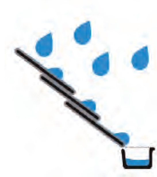
A simple rain water catchment showing transport from the roof to storage
