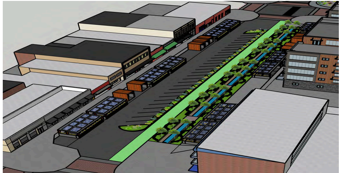
Alternative A would retain a one-way street throughout 4 blocks with road closure in the 1500 block. The 1300 block is shown in this view
