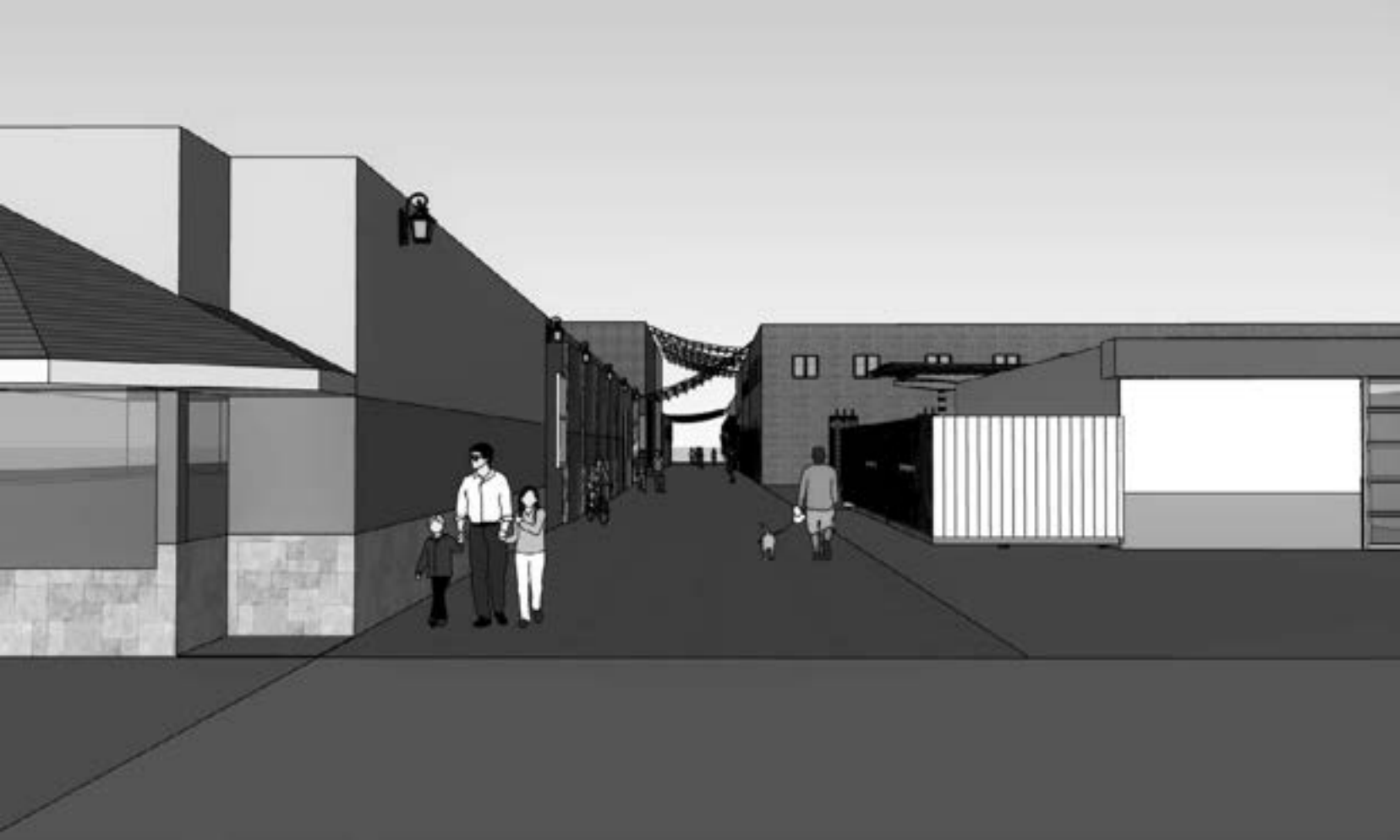
Figure 5.4.4: Southwest entrance of alley 10. This perspective view shows the absence of the dozens of small trash bins lining the alley currently, and you can see the consolidated trash area behind jiffy lube. The perspective also shows added lighting on the southeast side of the alley, and paving stone throughout the entire alley.
