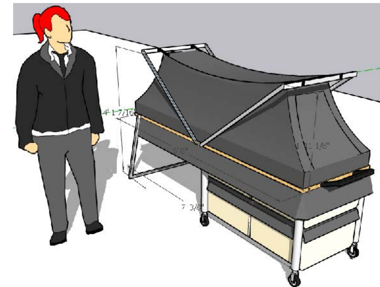
Figure 4.1: This bare bones version shows the drawers and folding logistics more clearly
