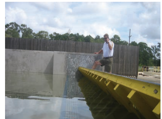
Figure 5.8 Demonstration of passive flood barrier on roadway (Floodbreak LLC)
