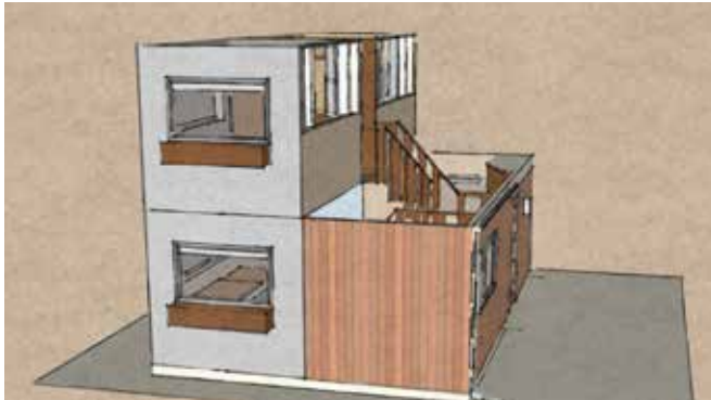
Step two: Place second story of home on first story.
