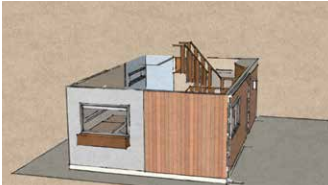
Step one: Set bottom two sections of home on foundation.
