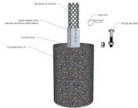
Figure 2. Placement of anchors supporting awning structures.
