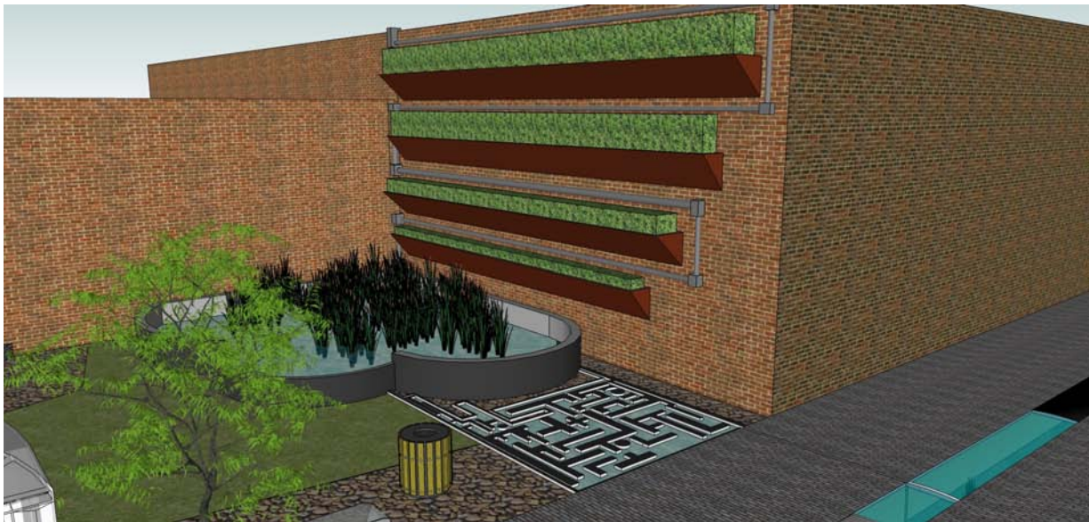
Living wall and water treatment system in the pocket park.
