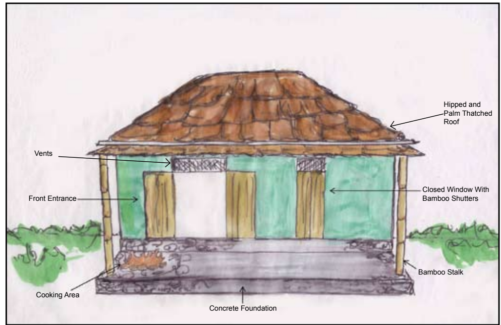
Front View of Shelter (refer to illustration on front chapter page for details)
