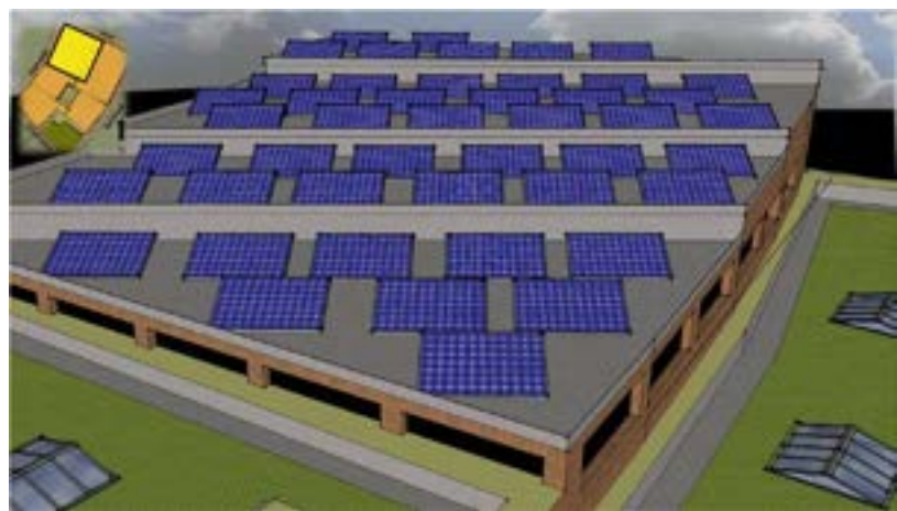
Figure 3.6: Photovoltaic panels mounted above fourth story parking garage.
