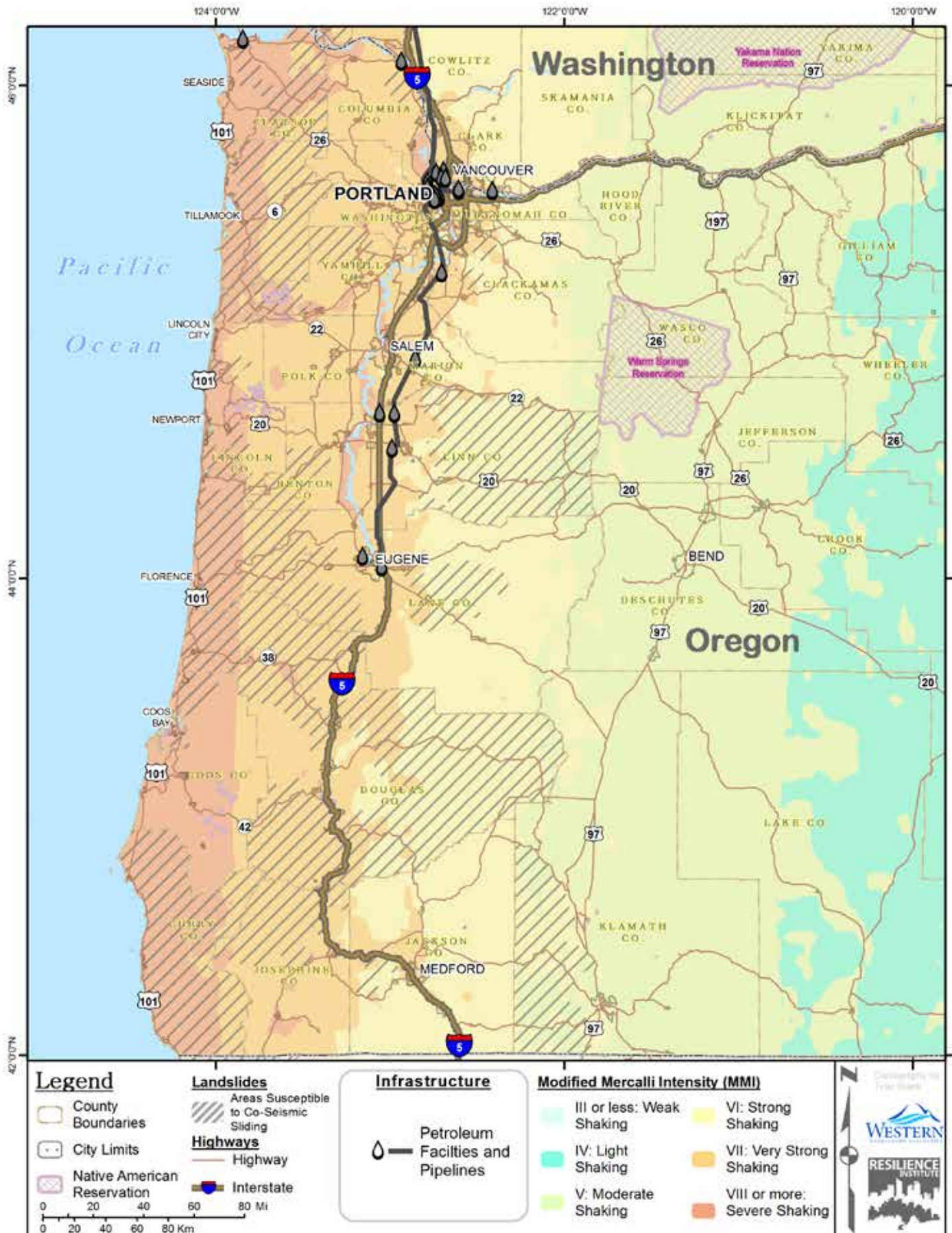
Figure 64. Oregon refined fuel facilities and pipelines in relation to shaking intensity and landslide potential
