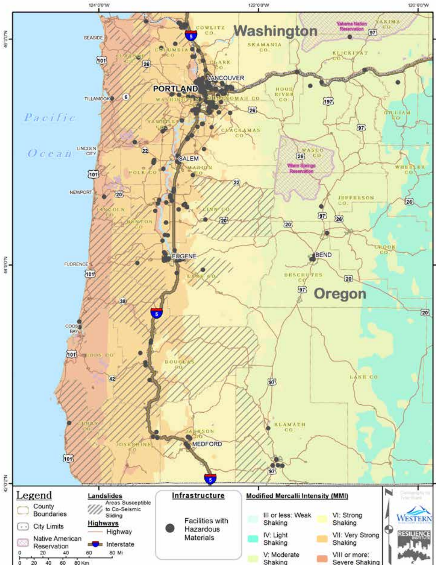
Figure 103. Oregon facilities with hazardous material in relation to shaking intensity and landslide potential
