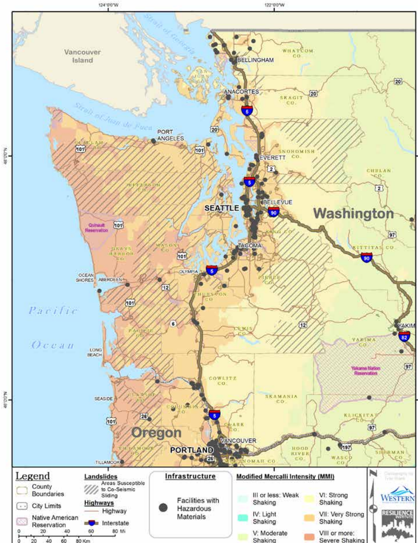
Figure 101. Washington facilities with hazardous material in relation to shaking intensity and landslide potential
