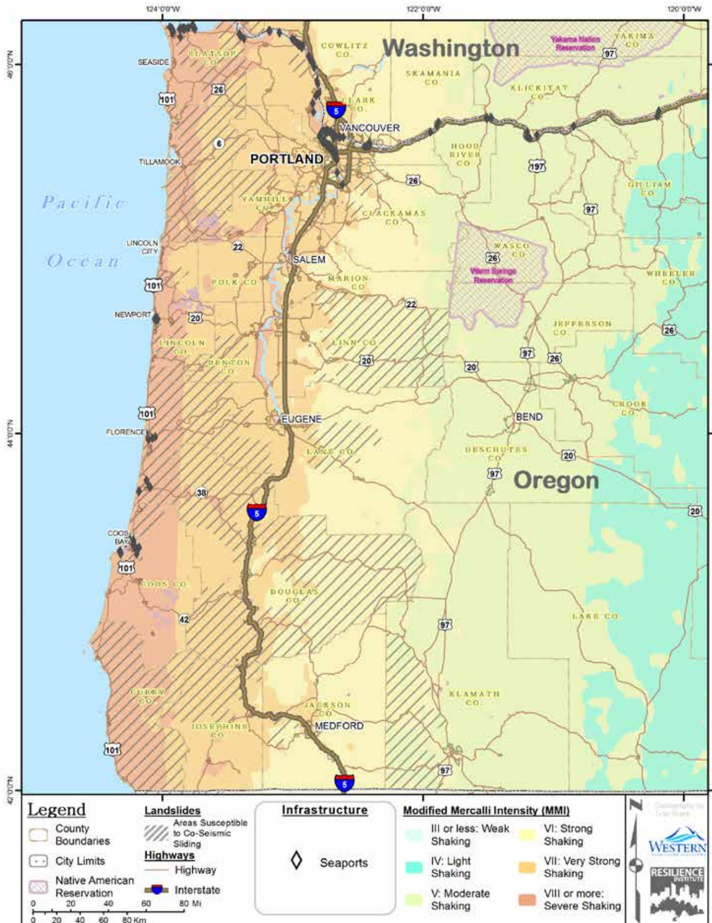
Figure 55. Oregon ports in relation to shaking intensity and landslide potential
