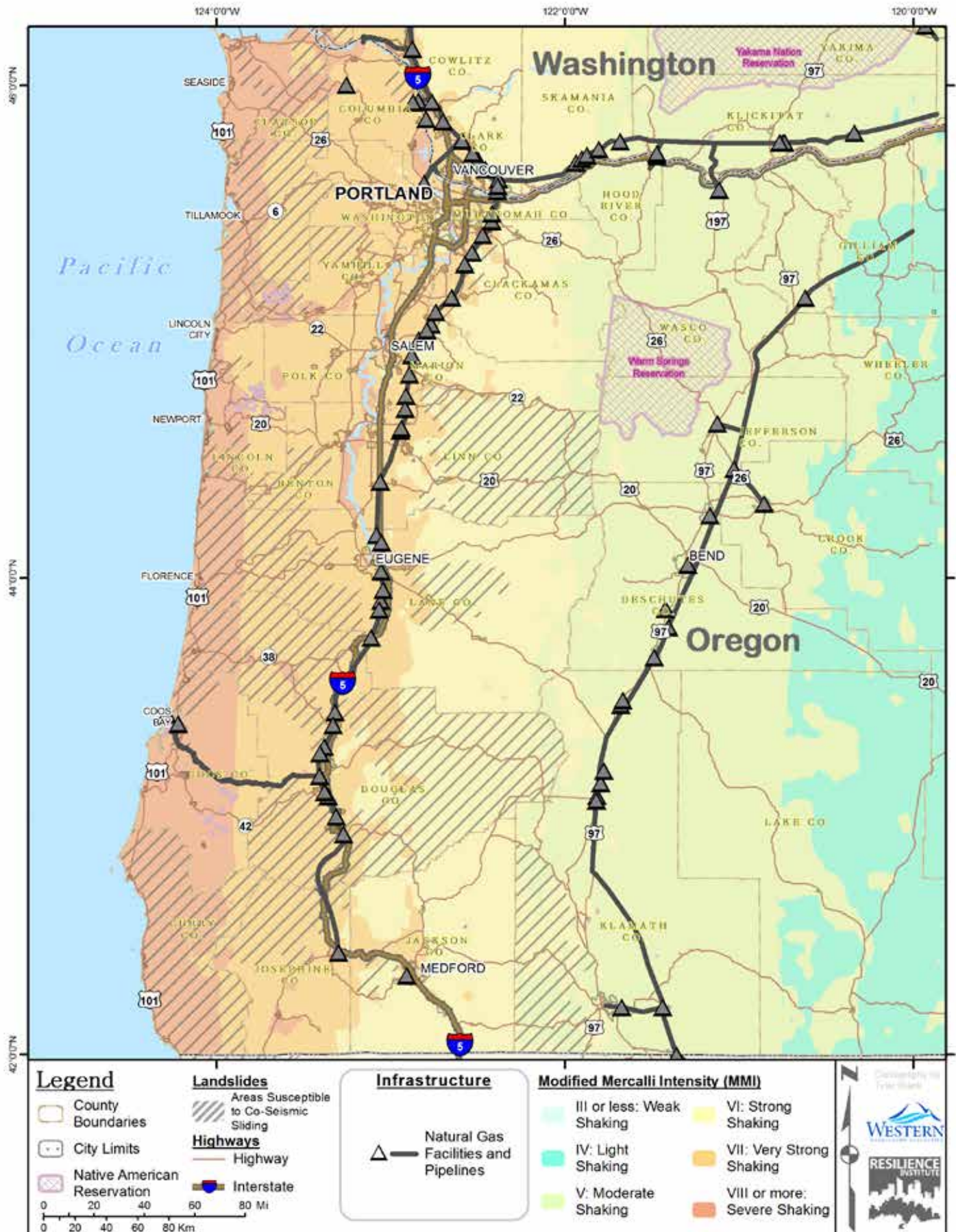
Figure 62. Oregon natural gas facilities and pipelines in relation to shaking intensity and landslide potential
