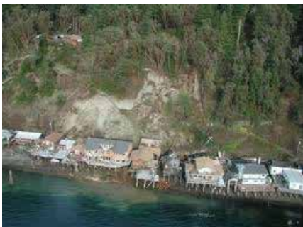
Figure 5. Earthquakes can trigger preexisting landslides. This could happen immediately or days to weeks later. The 2001 Nisqually earthquake triggered a landslide three days after the earthquake. The same hillside slid after the 1949 South Puget Sound earthquake. Photo: Dave Sherrod, USGS.
