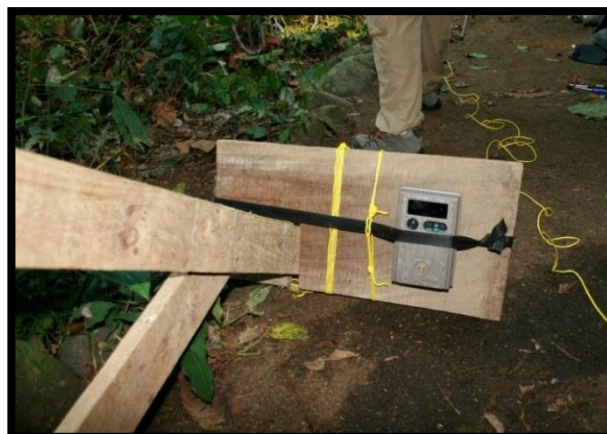
Photo 1. Camera Trap Mount.
